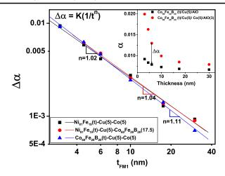
FIG. 1 (color online). Contributed Gilbert damping  $\Delta\alpha(t_{F1})=\alpha_{F2}(t_{F1})-\alpha_{\text{no}F2}(t_{F1})$  from the introduction of a second  $F_2$  interface in  $F_1(t_{F_1})/\text{Cu}(5 \text{ nm})[/F_2]/\text{Al}(3 \text{ nm})$  structures. Inset:  $\alpha_{\text{no}F2}(t_{F1})$  and  $\alpha_{F2}(t_{F1})$  for CoFeB layers.
