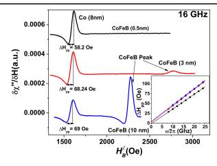
FIG. 2 (color online). Isolation of contribution to Gilbert damping in  $F_1/\text{Cu}/F_2(t_{F2})$ ,  $F_1 = \text{Co}(8\,\text{nm})$ ,  $F_2 = \text{CoFeB}t_{\text{CoFeB}}$ . Main panel: Derivative FMR spectra, 16 GHz,  $t_{\text{CoFeB}} = 0.5$ , 3.0, and 10.0 nm. Note the increase in linewidth for the Co resonance (low field) as a function of  $t_{\text{CoFeB}}$ . Inset: Separation of intrinsic and extrinsic damping for different  $t_{\text{CoFeB}}$ .
