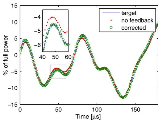
FIG. 2 (color online). Portion of a typical pulse shape showing the designed target shape (solid blue line), the initial attempt at implementing the pulse including systematic imperfections due to nonlinearities in pulse generation and amplification as well as finite bandwidth effects from the probe’s resonant circuit (red dots), and the corrected shape after the feedback protocol (green circles). Full power corresponds to nutation frequency of 80 kHz.
