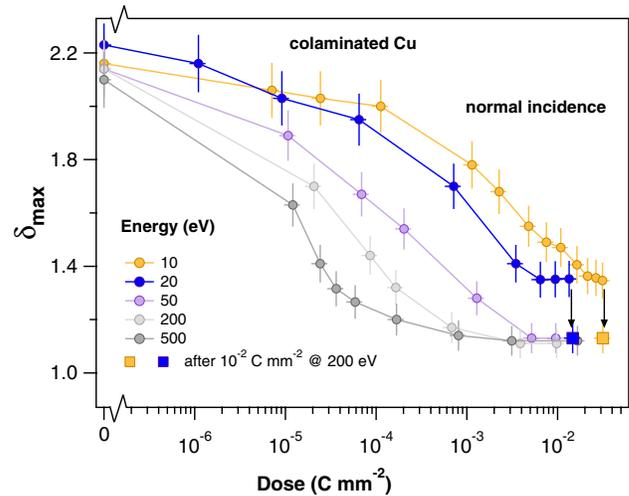
FIG. 1 (color online).  $\delta_{\max}$  as a function of the dose for different impinging electron energies at normal incidence on colaminated Cu of the LHC beam screen. The squares represent the  $\delta_{\max}$  values measured after an additional electron dose of  $1.0 \times 10^{-2}$  Cmm<sup>-2</sup> at 200 eV.
