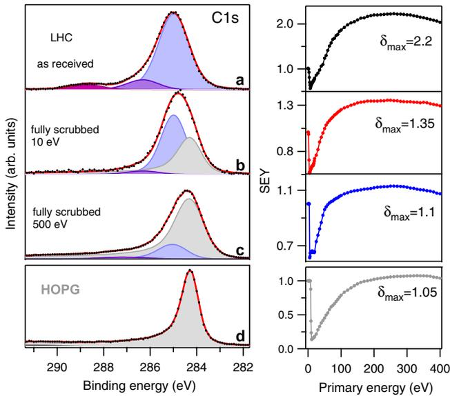
FIG. 2 (color online). C 1s XPS spectra and SEY curves measured on the LHC Cu sample: (a) “as received,” (b) after a dose of  $3 \times 10^{-2} \text{ C mm}^{-2}$  at 10 eV, (c) after a dose of  $3 \times 10^{-2} \text{ C mm}^{-2}$  at 500 eV, and (d) on a freshly cleaved HOPG surface.
