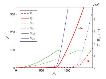
FIG. 2 (color online). Occupation of the *p* and *s* states in the steady state (left axis) and terahertz generation rate (right axis), as a function of pumping mode occupancy. The subscript 1 or 2 refers to the value of  $g^{(2)}(0)$  taken.  $W_g = 1$ ,  $W_G = 10$ ,  $1/\tau_s = 1000$ ,  $1/\tau_p = 5000$ , in units of  $W_g$ .
