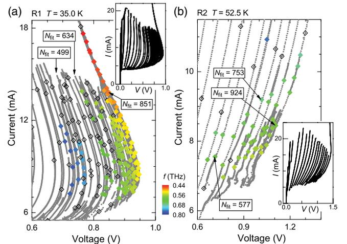
FIG. 2 (color online). Emission from IVC points at the color-coded frequencies was observed at the filled diamonds. No radiation was detected at the open diamonds. Arrows indicate the numbers  $N_{\text{fit}}$  of resistive junctions from fits to the Josephson relation. (a) R1. (b) R2. Insets: Full IVCs.
