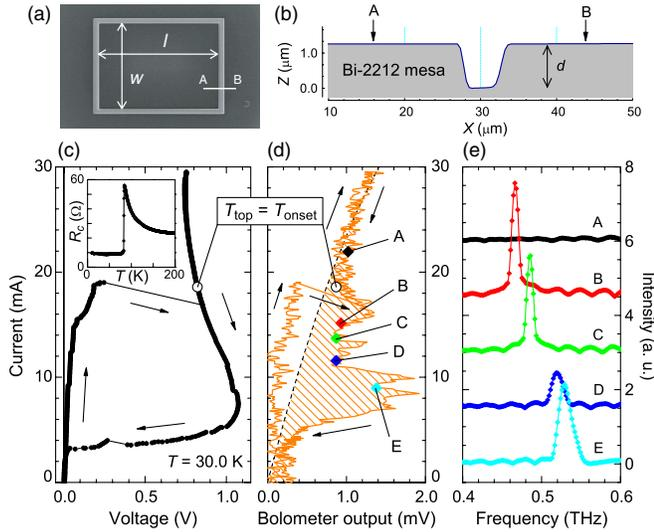
FIG. 1 (color online). R1 structure,  $c$ -axis resistivity, outermost-branch IVC, emission output, and frequency spectra. (a) Scanning ion microscope image. (b) Atomic force microscope image along  $A$ - $B$  in (a). (c) Outer-branch IVC. Inset:  $R_c(T)$ . (d) Plot of  $I(V_{\text{out}})$  corresponding to (c). Open circles:  $T_{\text{top}} = T_{\text{onset}} = 84.4$  K. (e) Spectral intensities from points  $A$ - $E$  in (d).
