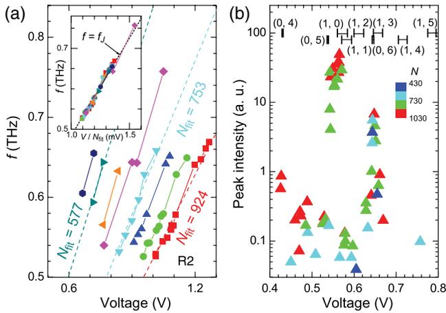
FIG. 4 (color online). Emission frequencies and intensities from  $R2$ . (a) Plots of  $f(V)$  for 8 branches in the  $R2$  IVCs. Dashed lines: Fits to  $f = f_J = (2e/h)V/N_{\text{fit}}$ . Inset: Plot of  $f(V/N_{\text{fit}})$  for all  $R2$  data. Dotted line:  $f = f_J$ . (b) Peak intensity on a logarithmic scale versus  $f$  for  $R2$ . Calculated  $f_{m,p}^c$  ranges are given at the top.  $N_{\text{fit}}$  values are color-coded.
