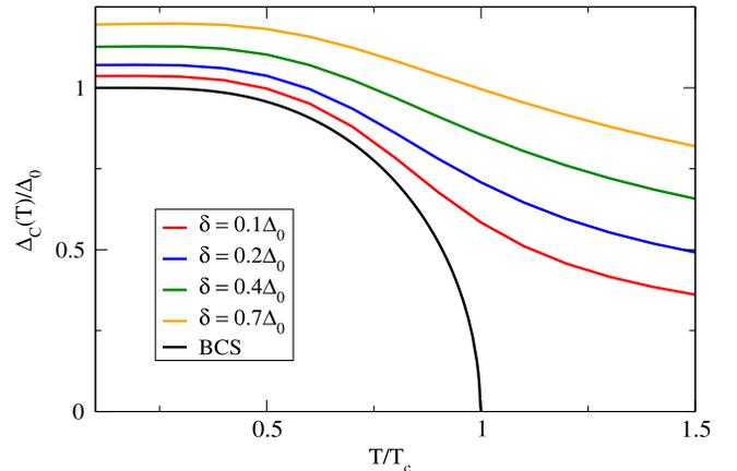
FIG. 1 (color online).  $\Delta_C(T)$  (6) for a constant spectral density  $\rho(\varepsilon) = 1/\delta$ .  $\Delta_C(T)$  combines thermal and quantum fluctuations. It reduces to the RPA (SPA) for  $T \ll T_C$  ( $T \gg T_C$ ).
