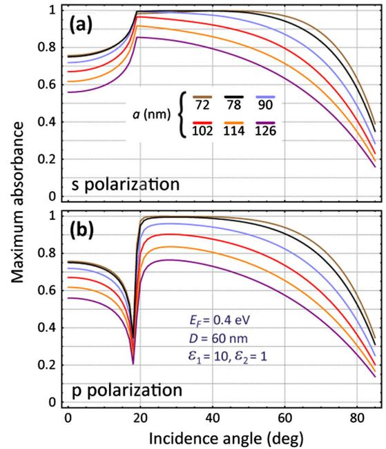
FIG. 3 (color online). Angular dependence of the peak absorbance for  $s$  (a) and  $p$  (b) polarization in arrays of graphene nanodisks [see Fig. 2(a)]. Each curve represents a fixed sample with parameters as shown by labels.
