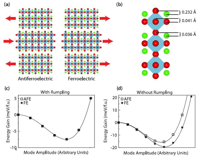
FIG. 4 (color online).  $\text{Sr}_4\text{Ti}_3\text{O}_{10}$  ground state under 1.1% tensile strain. (a) Schematic of ferroelectric (FE) and antiferroelectric (AFE) distortions. (b) Rumpling distortion (defined as the distance along [001] between cations and oxygens on the same layer). (c) Energy gain due to FE and AFE distortions in structures with rumpling. (d) The same as (c) except the rumpling distortion has been artificially set to zero.
