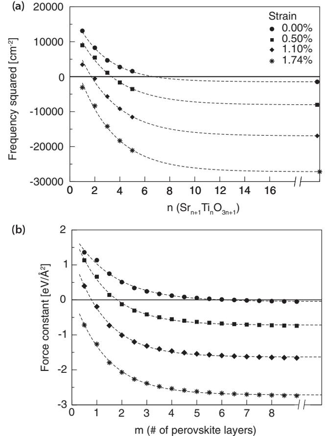
FIG. 3. (a) Ruddlesden-Popper,  $(\text{SrTiO}_3)_n(\text{SrO})$ : in-plane polar soft mode frequency squared versus layering number  $n$ . (b) Perovskite slab model,  $(\text{SrTiO}_3)_m$ : lowest in-plane polar interplanar force constant matrix eigenvalue versus thickness of SrTiO<sub>3</sub>. Strain values are given with respect to the lattice constant of SrTiO<sub>3</sub>. The lines are fits to exponentials.
