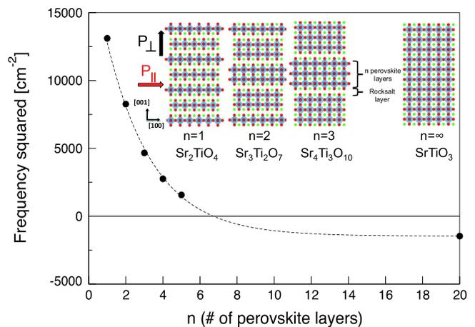
FIG. 1 (color online). (Inset) The Ruddlesden-Popper,  $\text{Sr}_{n+1}\text{Ti}_n\text{O}_{3n+1}$ , homologous series showing two possible polarization directions: in-plane,  $P_{\parallel}$ , and out-of-plane,  $P_{\perp}$ . (Main figure) Calculated in-plane polar phonon frequency as a function of  $n$  for a fixed in-plane lattice constant of  $\text{SrTiO}_3$ . (The dots are first-principles calculations; the curve is a fit to a single exponential.)
