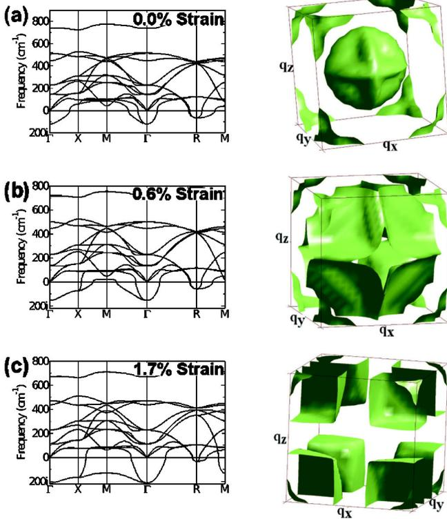
FIG. 2 (color online). Phonon dispersions of SrTiO<sub>3</sub> in its cubic ( $Pm\bar{3}m$ ) phase at (a) experimental volume, and under (b) 0.6% and (c) 1.7% isotropic tensile strain with respect to the experimental lattice constant. The corresponding  $\omega^2 = 0$  isosurfaces are shown next to each phonon dispersion curve.
