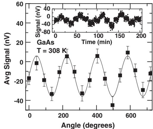
FIG. 2. Time-averaged signal from semi-insulating GaAs in zero magnetic field plotted against the change of angle between plane of incident polarization and the optical axis of the EOM. Inset shows the raw data acquired from the lock-in amplifier every 3 seconds for a total of  $\sim 3$  hours. The half-wave plate was rotated every  $\sim 10$  min to change the polarization axis. The solid line is a sinusoidal fit to the data.
