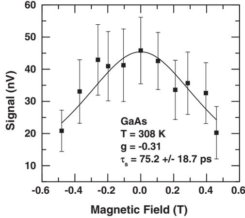
FIG. 3. Dependence of output signal (peak-to-peak value of the sinusoidal fit shown in Fig. 2) in GaAs on a magnetic field applied parallel to sample surface. Sample temperature was slightly higher than room temperature due to the high power laser beam. The data were fitted to the Hanle equation to extract the spin relaxation lifetime of  $75.2 \pm 18.7$  ps.
