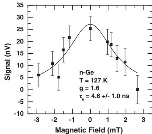
FIG. 5. Dependence of output signal (peak-to-peak value of the sinusoidal fit shown in Fig. 4) in Ge at  $127 \text{ K}$  on a magnetic field applied parallel to sample surface. Note the magnetic field scale compared to Fig. 3. The data was fitted to the Hanle equation to extract the spin relaxation lifetime of  $4.6 \pm 1.0 \text{ ns}$ .
