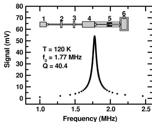
FIG. 1. Frequency response of rf pickup coil as measured by the rf lock-in amplifier, when excited by a current carrying coil in place of the sample. Inset shows experimental setup: (1) laser, (2) linear polarizer, (3) half-wave plate, (4) EOM, (5) rf coil with sample inside, (6) cryostat.
