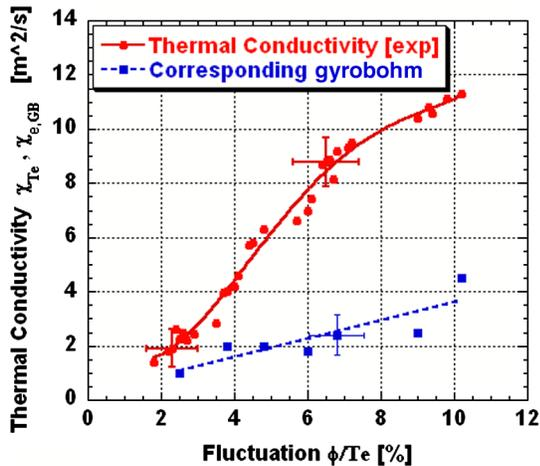
FIG. 4 (color online). Experimental scaling of electron thermal conductivity versus the potential fluctuation level and the corresponding gyrobohm diffusion coefficient.
