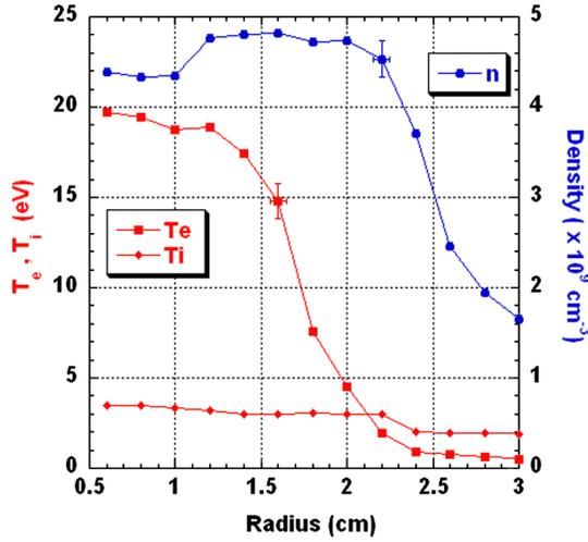
FIG. 2 (color online). Radial profiles of electron and ion temperature and plasma density.
