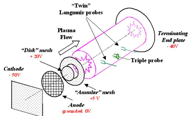
FIG. 1 (color online). Scheme of the CLM and electron heating method.
