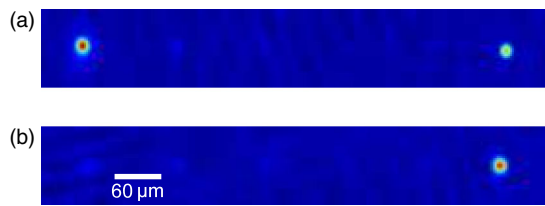
FIG. 2 (color online). (a) Absorption image of the cloud after the application of a 30\hbar k SB-LMT beam splitter. The beam splitter consists of five sequential 6\hbar k pulses (one \pi/2 pulse, four \pi pulses). The image is taken after 4 ms time-of-flight from the application of the first pulse, corresponding to a wave packet separation of 600\text{ }\mu\text{m} . The faint spots between the two main wave packets arise from pulse inefficiency due to imperfections. (b) Image of the cloud after the application of five consecutive 6\hbar k \pi pulses, effectively forming a 30\hbar k SB-LMT \pi pulse. Each 6\hbar k \pi pulse has an efficiency of 94%, corresponding to a total efficiency of \sim 73\% for the five pulse sequence. False color red corresponds to a higher atom density [33]. The images in this figure have been rotated by 90^\circ .
