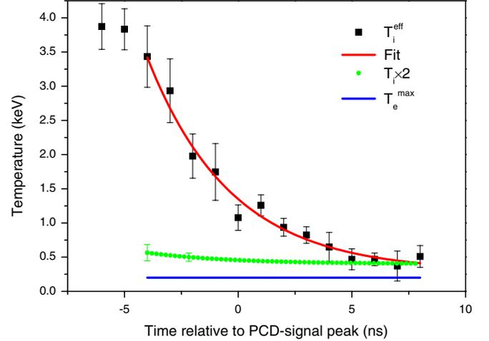
FIG. 2 (color online). The measured ion effective temperature, obtained from the measured line shapes, where each data point is an average of 2–5 identical discharges, together with the true ion temperature, calculated using Eq. (2).
