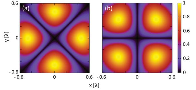
FIG. 1 (color). The distributions of the Lorentz invariants (a)  $|\langle \mathcal{F} \rangle|$  and (b)  $|\langle \mathcal{G} \rangle|$  of the focused laser beam in the focal plane for  $\theta = 100^\circ$ . The  $x$  and  $y$  axes are expressed in units of the laser wavelength  $\lambda$ . The Lorentz invariants are normalized to the peak value.
