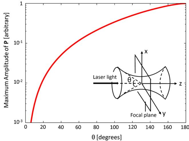
FIG. 3 (color online). Angular aperture dependence of the maximum amplitude of the polarization  $\mathbf{P}$  in the focal plane under a fixed laser intensity, and geometric configuration of the incident laser light. The maximum amplitude of  $\mathbf{P}$  is equal to that of the magnetization  $\mathbf{M}$ . The amplitude is normalized to the value for  $\theta = 180^\circ$ .
