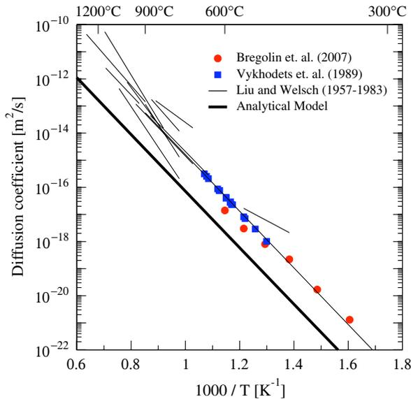
FIG. 3 (color online). Analytical results and experimental data of oxygen diffusivity in  $\alpha$  titanium. We compare our analytical DFT model (bold line) to experimental data from the literature survey by Liu and Welsch [25] (thin lines), and experiments by Bregolin [26] and Vykhodets [27] (symbols).
