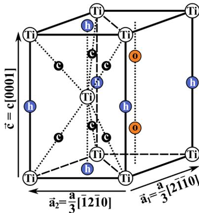
FIG. 1 (color online). Wyckoff positions [22] and relative energies for oxygen interstitial sites in  $\alpha$  titanium. The interstitial site energy  $\Delta E$  is reported relative to the octahedral site energy. The geometry of each site is characterized by the nearest neighbor distance after relaxation,  $R_{nm}$ , with coordination number  $Z$ . Titanium atom sites are in white, while oxygen interstitial sites are in orange (octahedral), blue (hexahedral), and black (crowdion).
