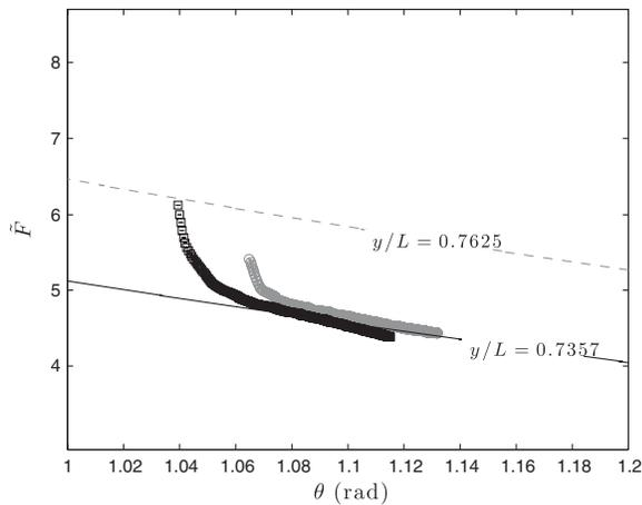
FIG. 4. Evolution of the dimensionless force  $\tilde{F}(\theta)$  measured for two different runs ( $\circ$ ). Experiments were performed in Mylar sheets of thickness  $h = 0.35$  mm at the same imposed initial spacing  $y/L = 0.7625$ . The predictions of the elastica for the experimentally imposed spacing (dashed line) and for  $y/L = 0.7357$  (continuous line) are also shown.
