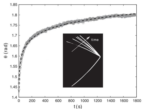
FIG. 1. Uncontrolled experiment: time evolution of the angle of a crease made in a rectangular sheet of Mylar of thickness 0.35 mm (see the inset). The dashed line is a logarithmic fit  $\theta(t) = a \log(t) + b$  with  $a = 0.055$  and  $b = 1.392$ . Inset: Superimposed images of the sheet during the relaxation process.
