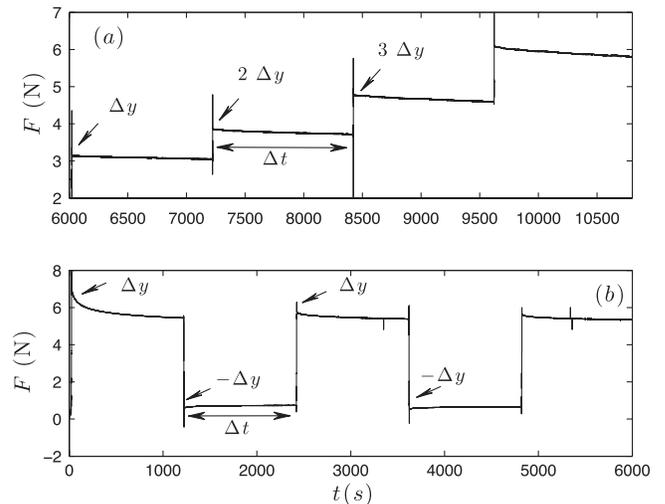
FIG. 5. Experimental runs showing the two protocols followed for the characterization of the force relaxation. (a) The fold spacing is increased periodically by an increment  $\Delta y$  starting from an initial spacing  $y_0$ . (b) The fold spacing is alternately increased and decreased by an increment  $\Delta y$ . The time interval  $\Delta t$  between two successive events and  $\Delta y$  are the control parameters of the experiment.
