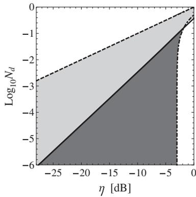
FIG. 2. Comparison between criterion based on negativity of the Wigner function (white area below dash-dotted curve) and the proposed criterion (area below solid curve) for the single photon generated by the emitter in a weak coupling regime. See text for details.
