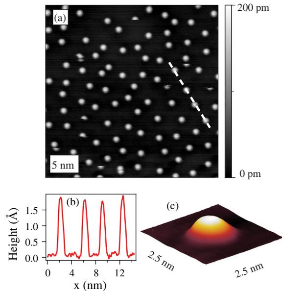
FIG. 2 (color online). Topographic image of the graphite surface after the deposition of potassium, showing isolated potassium atoms. The tunneling bias and current are  $-2$  V and 5 pA. (b) The height profile is taken along the dotted line drawn in (a). (c) Landscape (full height 200 pm) of a single potassium atom.
