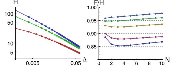
FIG. 3 (color online). (Left): Log-log plot of the QFI for optimized pure input Gaussian states as a function of the noise parameter  $\Delta$  for different values of the average photon number. From bottom to top:  $N = \{2, 5, 10\}$ . (Right): Ratio between the FI of homodyne detection on coherent states and the corresponding QFI, as a function of the number of photons of the probe states and for different values of  $\Delta$ . From bottom to top:  $\Delta^2 = \{0.5, 1.0, 1.5, 2.0, 5\}$ .
