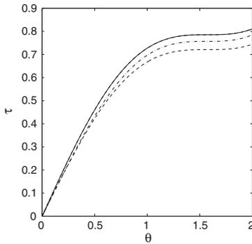
FIG. 3. Variation of the actual time  $\tau$  with respect to the timelike variable  $\theta$  for three cases: (i)  $\epsilon = 0 = \eta$ ;  $t_c = 0.785$  (solid line); (ii)  $\epsilon = 0.1$ ,  $\eta = 0$ ;  $t_c = 0.721$  (dotted line); and (iii)  $\epsilon = 0.1$ ,  $\eta = 0.03$ ;  $t_c = 0.757$  (dash-dotted line).
