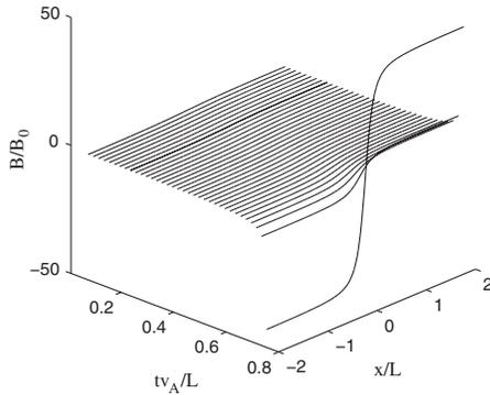
FIG. 1. Normalized magnetic field evolution with finite dispersion  $\epsilon = 0.1$  and dissipation  $\eta = 0.03$ . The figure shows that neither finite dispersion nor resistivity can stop the magnetic field singularity. The latter has merely a delaying effect on the collapse time, which occurs at  $t_c = 0.757$ , the time measured in Alfvén transit time.
