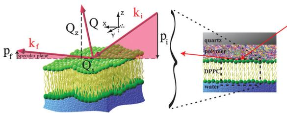
FIG. 1 (color). Geometry for an OSS event. Neutrons penetrate the quartz substrate and polymer cushion to reach the buried membrane (right). The thickness of the bilayer (38 Å) as compared to the polymer (200–900 Å) has been greatly exaggerated for the sake of clarity. If the incident and outgoing angles are unequal, then the momentum transfer vector  $Q$  has components perpendicular  $Q_z$  and parallel  $Q_x$  to the scattering interface.
