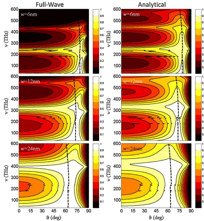
FIG. 2 (color online). Angular transmission spectra for a grating thickness  $l = 200$  nm and period  $d = 96$  nm. The slit width is indicated in each panel. Fourier modal method simulations (left) are compared with analytical results (right). The dashed line indicates the plasmonic Brewster angle condition.
