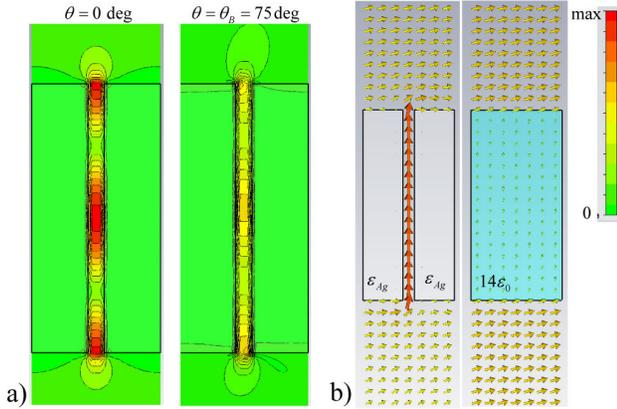
FIG. 4 (color online). (a) Electric field distribution  $E_x$  on the  $E$  plane for  $l = 400$  nm,  $d = 192$  nm, and  $w = 24$  nm at  $f = 395$  THz for normal incidence (left) and incidence angle  $\theta_B = 75^\circ$  (right). (b) Power flow distribution at the Brewster angle (left) and comparison with an equivalent dielectric etalon with  $\epsilon = 14\epsilon_0$ . In each panel, the fields are normalized to the same scale.
