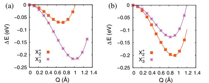
FIG. 4 (color online). Effect of epitaxial strain on the unstable zone-boundary modes in  $\text{Ca}_3\text{Mn}_2\text{O}_7$ . Change in energy per formula unit with regard to paraelectric  $I4/mmm$ , as a function of the amplitudes of the  $X_3^-$  and  $X_2^+$  modes under (a) 1.5% tensile and (b) 1.5% compressive biaxial strain. The lines are a guide to the eye (similar results were also found for  $\text{Ca}_3\text{Ti}_2\text{O}_7$ ).
