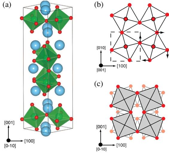
FIG. 1 (color online).  $\text{Ca}_3\text{Mn}_2\text{O}_7$  structure and rotation distortions. (a) The  $A2_1am$  ferroelectric ground state structure. Large (blue) spheres correspond to Ca ions. (b) Schematic of the atomic displacements corresponding to the  $X_2^+$  rotation. The dashed square denotes the unit cell of the  $I4/mmm$  parent structure. (c) Schematic of the  $X_3^-$  tilt mode. All axes refer to the coordinate system of the  $I4/mmm$  parent structure.
