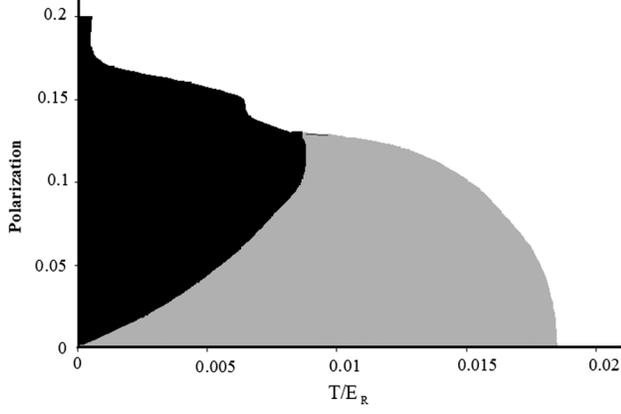
FIG. 1. The phase diagram of the imbalanced Fermi gas in a 2D lattice (FF = black, Sarma = gray, normal = white). The total filling factor is  $f = 0.5$ . The interaction strength is  $U/J = 2.64$ , where  $J/E_R = 0.0783$ . For  ${}^6\text{Li}$  atomic Fermi gas and  $\lambda = 1030$  nm,  $E_R = 1.293 \times 10^{-11}$  eV.
