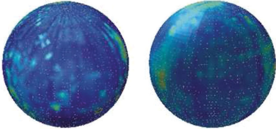
FIG. 2 (color). Topographic maps of the surface layer thickness. Left AVO28-S5; right AVO28-S8. The rainbow colors range from 2.0 nm (blue) to 4.5 nm (yellow).
