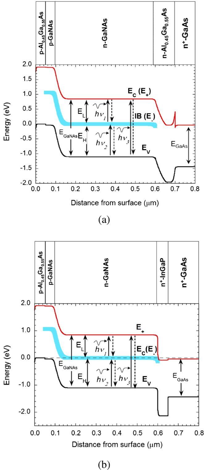
FIG. 1 (color online). (a) The structure and band diagram of a BIB device with the intermediate band (IB) disconnected from the contacts. Transitions generating electron-hole pairs utilizing the IB are denoted as  $h\nu_1$ ,  $h\nu_2$ . The transitions from VB to CB are represented by  $h\nu_3$ . (b) The structure and the band diagram of an UIB device with the IB connected to the backside contact. The electron affinity values for AlGaAs and InGaP are 3.63 and 4.1 eV, respectively.
