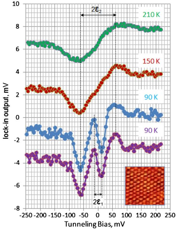
FIG. 1 (color online). Inelastic tunneling spectra obtained on Au(111) surface at three different sample temperatures: 210 K (upper curve), 150 K (middle curve), and 90 K (two lower curves: obtained at different portions of sample surface). The curves are offset along the vertical axis. Inset:  $3 \times 3 \text{ nm}^2$  atomically resolved STM image of Au(111) sample. Obtained at 90 mV sample bias and 0.5 nA current.
