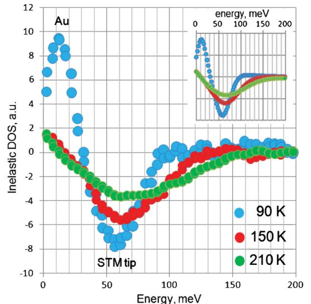
FIG. 2 (color). Temperature-dependent IETS density of states obtained from spectra in Fig. 1 by averaging the contributions for positive and negative tunnel bias. Inset: Gaussian fit curves.
