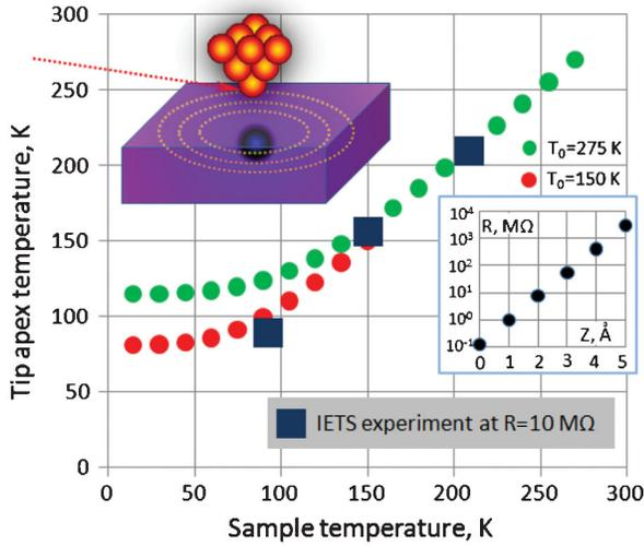
FIG. 4 (color). The dependence between STM tip apex temperature and sample temperature predicted by model of “thermal mirage.” Green and red curves correspond to tip “bulk” temperatures of 275 and 150 K, respectively. Inset: the dependence of vacuum gap resistance on tip vertical displacement for the Au(111) sample. The IETS measurements were made at 10 MΩ resistance.
