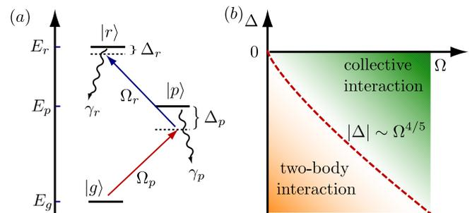
FIG. 1 (color online). (a) Setup for the ground state dressing with the Rydberg level  $|r\rangle$  via the intermediate  $|p\rangle$  state with the corresponding Rabi frequencies and detunings. (b) Diagram showing the crossover from the two-body interaction potential into the regime with a collective many-body interaction. The crossover line is determined by  $|\Delta| \sim \Omega^{4/5}$  (red dashed line), which preempts the condition of weak dressing  $\Omega \lesssim |\Delta|$ .
