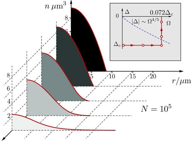
FIG. 3 (color online). Density profile  $n(r)$  for a Bose-Einstein condensate of  $^{87}\text{Rb}$  atoms in a harmonic trap  $\omega = 100$  Hz with background scattering length  $a_s = 5.7$  nm for increasing influence of the Rydberg dressed interaction. The inset shows the path within the parameter space for increasing interaction strengths.
