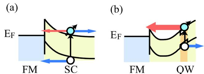
FIG. 1 (color online). Schematic diagram of photocurrent transmission at (a) an FM/*n*-SC interface and (b) an FM-SC QW (e.g., Fe/GaAs QW) interface. The red arrow denotes the spin-dependent photocurrent, while the blue arrows express spin-independent photocurrent contribution.
