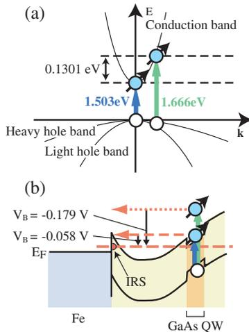
FIG. 4 (color online). Schematic diagram of (a) the excitation process in a QW and (b) spin-dependent transmission process of excited electrons at the Fe/GaAs QW interface. The blue and green arrows represent the excitation at 1.503 and 1.666 eV, respectively. The red arrows (dotted and dashed) express the transmission of spin-polarized electrons.  $V_B = -0.179$  and  $-0.058$  V denote the applied bias voltage. The dashed line is the energy level where the localized states are formed.
