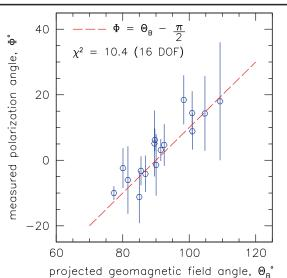
FIG. 4 (color). Plane of polarization of UHECR events compared to the angle of the magnetic field local to the event and Lorentz force expectation (red line). Reflected events are corrected for surface Fresnel coefficients. Angles are from the horizontal.
