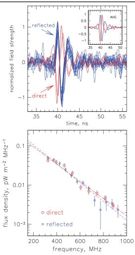
FIG. 3 (color). Top panel: Overlay of the 16 UHECR event  $H_{pol}$  pulse shapes, showing the two direct events (red) and 14 reflected events (blue) with inverted phase. Inset: Average pulse profile for all events. Bottom panel: Flux density for both the averaged direct and reflected events, along with fits to an exponential. Errors at low frequency are primarily due to systematic uncertainty in the antenna gains, and to thermal noise statistics at higher frequencies.
