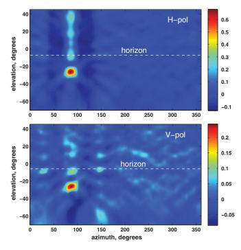
FIG. 1 (color). Interferometric map of relative correlated intensity in  $H_{\rm pol}$  (top panel) and  $V_{\rm pol}$  (bottom panel) for event 3 623 566, which occurred in a region of Antarctica where the geomagnetic inclination gave an appreciable  $V_{\rm pol}$  component. Map details are covered elsewhere [20].
