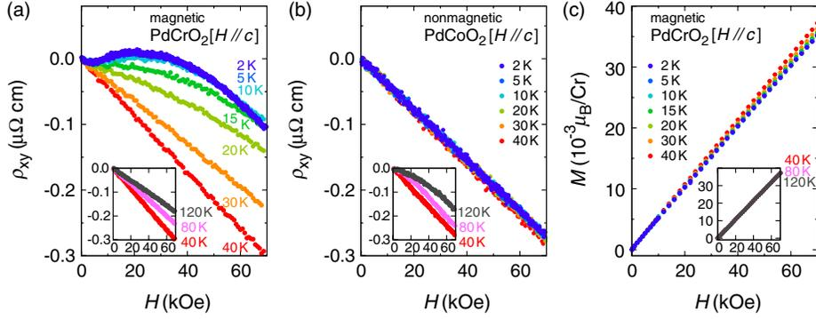
FIG. 1 (color online). Field dependence of the Hall resistivity  $\rho_{xy}$  for (a) PdCrO<sub>2</sub> ( $T_N = 37.5$  K) and for (b) nonmagnetic PdCoO<sub>2</sub>. (c) Field dependence of the magnetization  $M$  for PdCrO<sub>2</sub>. Insets represent data at temperatures above 40 K. On cooling below  $T^* \approx 20$  K,  $\rho_{xy}$  of PdCrO<sub>2</sub> strongly deviates from the linearity and exhibits a hump to positive values at around 10–30 kOe.
