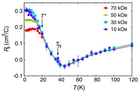
FIG. 3 (color online). Temperature dependence of  $R_S(H, T)$  represented by Eq. (2).  $R_S(H, T)$  does not depend on the magnetic field at temperatures above  $T^* \approx 20$  K, whereas below  $T^*$  it is field dependent, indicating the appearance of UAHE.
