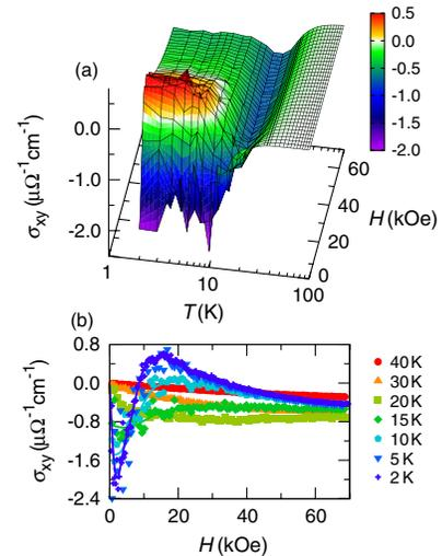
FIG. 4 (color online). (a) 3D representation of the overall field and temperature dependence of the Hall conductivity  $\sigma_{xy}$ . (b) Field dependence of  $\sigma_{xy}$  at temperatures below 40 K. From a point of view based on the scalar spin chirality mechanism, the fictitious field has the opposite sign to the applied magnetic field in the red region in (a).
