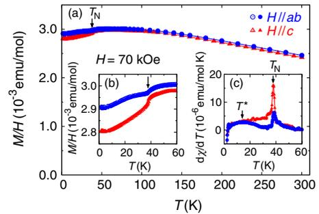
FIG. 2 (color online). (a) Temperature dependence of the magnetic susceptibility of single-crystalline PdCrO<sub>2</sub> for fields along the  $c$  axis ( $\chi_c = M_c/H$ ) and in the  $ab$  plane ( $\chi_{ab} = M_{ab}/H$ ) at 70 kOe. (b) Details of the anisotropy below  $T_N$ . Open (closed) symbols represent data in the field cooling (zero-field cooling) condition. (c) Temperature derivative of  $\chi_c$  and  $\chi_{ab}$ .
