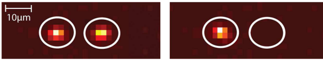
FIG. 4 (color online). Left: Fluorescence image of two \text{Ba}^+ ions. Right: Fluorescence of one ^{138}\text{Ba}^+ next to an unknown dark ion. We infer the existence of the dark ion from the position of the \text{Ba}^+ .
