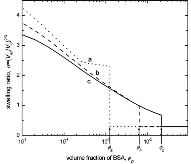
FIG. 3. Dependence of the swelling ratio  $\alpha$  on the protein volume fraction  $\phi_P$  for different salt concentrations  $n_s = 10^{-6}$  (a),  $5 \times 10^{-6}$  (b), and  $10^{-5}$  (c).  $\phi_i$  is the critical protein concentration for inducing the folding transition into a compact state.
