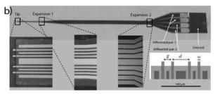
FIG. 1. (a) Schematic of probe and small electron beam in the LAPD device. (b) Highly magnified photograph of the electric field MEMS microprobe. The conductor is made from gold and the insulating material is polyimide. The dimensions are  $w=10~\mu\text{m}$ ,  $g=30~\mu\text{m}$ , and  $d=70~\mu\text{m}$ . The wires are coaxial and tapered in their expansion regions to maintain a 50  $\Omega$  impedance [9].
