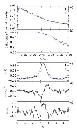
FIG. 2 (color online). Power spectrum (a) and coherence (b) for potential time series on two field-aligned probes separated by  $2.3\lambda_{De}$ . A solitary potential pulse (c), its bipolar electric field (d), and estimated charge density perturbation (e). In this and all other figures the parameters used for normalization correspond to the unperturbed state before beam injection.
