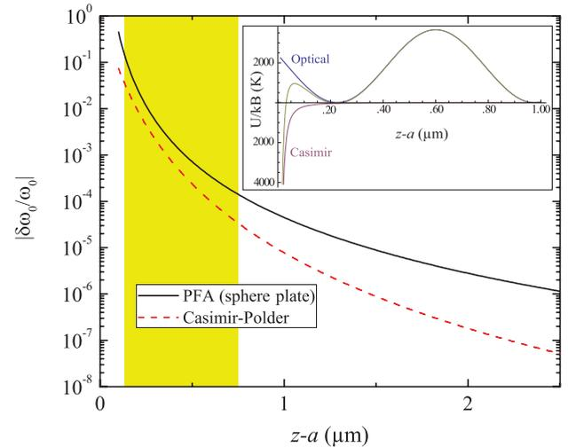
FIG. 2 (color online). Fractional frequency shift due to Casimir interaction of microspheres of radius  $a = 150$  nm at distance  $z$  from the gold surface. The PFA is expected to be valid at short distances, while the Casimir-Polder form is expected at large distances, and the transition region is shown as a shaded area. Inset: Optical and Casimir contributions to the cavity trapping potential.
