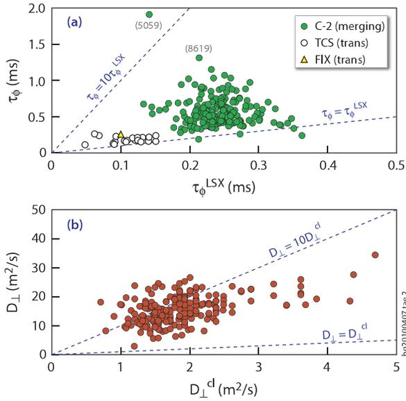
FIG. 7 (color online). (a) Magnetic flux decay time,  $\tau_\phi$ , versus the LSX scaling for conventional  $\theta$ -pinch formed FRCs,  $\tau_\phi^{\text{LSX}}$ , and results from recent FRC translation experiments, TCS [5] and FIX [3]; (b) diffusivities,  $D_\perp$ , derived from  $\tau_\phi$ , versus classical diffusivities,  $D_\perp^{\text{cl}}$ , for the well-centered merging FRCs in C-2.
