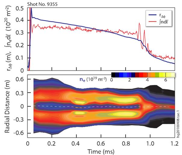
FIG. 6 (color online). Time evolution of the excluded flux radius  $r_{\Delta\phi}$  and the line-integrated density  $\int n_e dl$  at  $r = 3.3$  cm obtained from a six-channel integrated CO<sub>2</sub>/HeNe interferometer system (top), and contour of the electron density  $n_e(r)$  deduced from the interferometer measurements using the Abel inversion technique (bottom).
