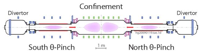
FIG. 1 (color online). Schematic of the C-2 device.
