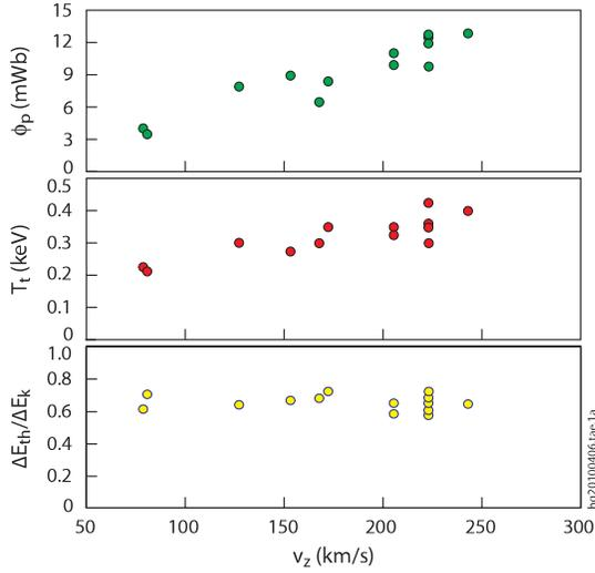
FIG. 4 (color online). Effect of dynamic translation speed. The data are obtained right after merging ( $\sim 40 \mu s$ ) of the FRC from a series of reproducible and well-controlled discharges with the same magnetic configurations and gas fuelling rates. The translation speed is varied by energizing the  $\theta$ -pinch coils at various different times during the initial formation process. Conservation of particle number is assumed.
