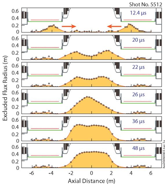
FIG. 2 (color online). Evolution of the excluded flux radius in C-2 obtained from a series of external diamagnetic loops at the two  $\theta$ -pinch formation sections and magnetic probes embedded inside the central metal confinement chamber. Time is measured from the instant of synchronized field reversal in the  $\theta$  pinch sources, and distance  $z$  is given relative to the center of the confinement chamber.
