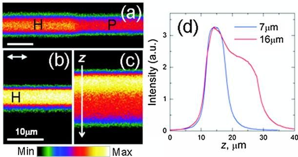
FIG. 4 (color online). Vertical FCPM views of hybrid aligned wedges with mixture  $A$ ; (a) vertical boundary between  $H$  and  $P$  states,  $d = 10 \mu\text{m}$ ; (b) homeotropic thin,  $d = 7 \mu\text{m}$  and (c) hybrid thick,  $d = 16 \mu\text{m}$ , parts of the same wedge and comparison of their fluorescent profiles (d). The double arrow in (b) shows light polarization  $\mathbf{P}$ .
