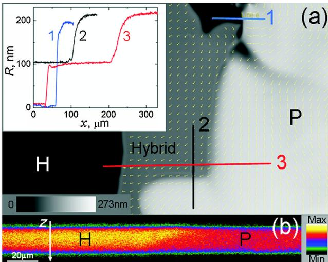
FIG. 2 (color online).  $H$ - $P$  transition in the mixture  $A$  viewed as (a) a grey scale map of  $R$  in  $(x, y)$  plane of the cell ( $d \approx 11 \mu\text{m}$ ) and as a variation of  $R$  along the lines 1, 2, and 3 (inset); (b) a FCPM vertical cross section of a cell with a tilted boundary.
