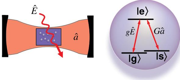
FIG. 1 (color online). Schematic diagram of the system: A quantized probe field  $\hat{E}$  interacts with an ensemble of  $\Lambda$ -type atoms driven by a cavity mode  $\hat{a}$  (left) in a Raman type coupling scheme (right).
