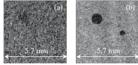
FIG. 2. Conventional GI (a) and DGI (b) of two totally absorbing particles 820 and 400  $\mu\text{m}$  in diameter, retrieved after  $m = 10^4$  averages. The number of speckles in the beam was  $N_{\text{speckle}} \sim 4590$ .
