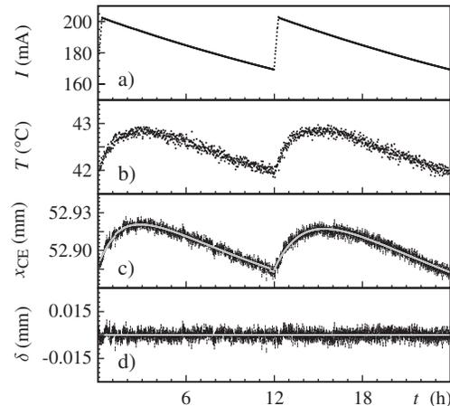
FIG. 3. Time evolution over a day of (a) ESRF beam intensity, (b) tagging-box temperature, (c) CE position and fitted curve [Eq. (5)], and (d)  $\delta = x_{CE} - x_{\text{fit}}$ . The error bars on position measurements are directly given by the CE fit.
