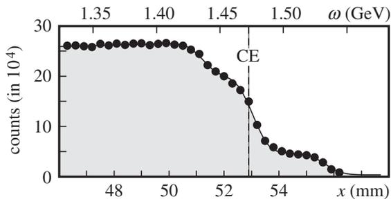
FIG. 2. Si  $\mu$ -strip count spectrum near the CE and the fitting function (see text) vs position  $x$  and photon energy  $\omega$ . The three edges corresponding to the lines 364, 351, and 333 nm are clearly visible. The CE position  $x_{CE}$  is the location of the central line and is measured with a typical accuracy of  $3 \mu\text{m}$ .
