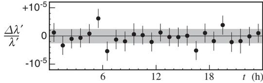
FIG. 4. Full set of data folded modulo a sidereal day (24 bins). The error bars are purely statistical and agree with the dispersion of the data points ( $\chi^2 = 1.04$  for the unbinned histogram). The shaded area corresponds to the region of nonexcluded signal amplitudes.
