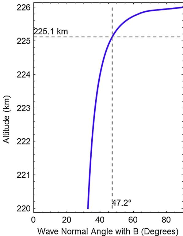
FIG. 3 (color online). Computed wave normal angle in the plasma for an oblique,  $O$ -mode plane wave launched from the ground at 4.2 MHz. The plasma layer profile for the computation is derived from the ionogram taken at the time of the HAARP experiment shown in Fig. 2.
