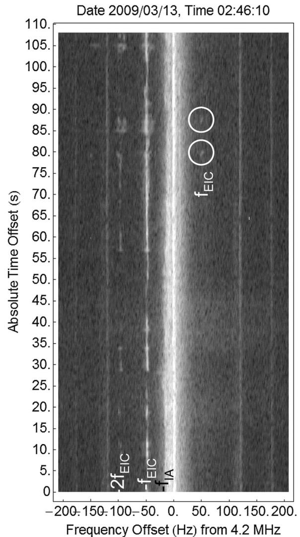
FIG. 2. Spectrogram of the stimulated Brillouin scatter lines for a pump wave beam offset 21.4 degrees from the magnetic field direction.
