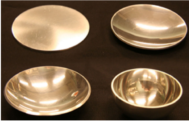
FIG. 2 (color online). Aluminum shells used in the experiment. From left to right, the opening angle is \theta_0 = 0^\circ , 25^\circ , 52^\circ , and 90^\circ .
