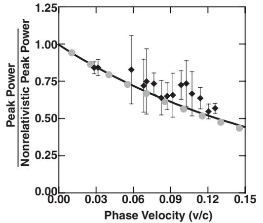
FIG. 3. The measured peak powers in the redshifted feature are divided by the calculated peak powers [Eq. (3), diamonds] and are plotted as a function of phase velocity. The electron temperature ranged from 85 to 720 eV. Data in perfect agreement with the nonrelativistic form factor would have a value of unity. The ratio of the relativistic peak power (solid line) and the corrected nonrelativistic peak power [Eq. (2), gray circles] divided by the nonrelativistic peak power are shown.
