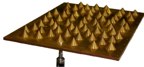
FIG. 1 (color online). Photograph of one of the two scattering arrangements used. The platform has width 260 mm and length 360 mm. Each cone has diameter 25 mm and height 15 mm. The probe antenna is fixed in a horizontally movable top plate located 20 mm above the bottom (not shown).
