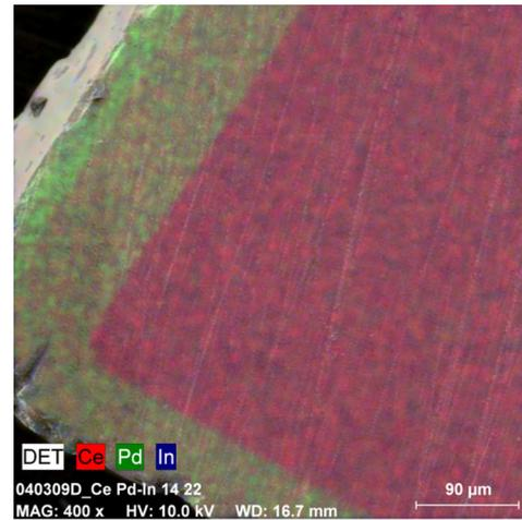
FIG. 1 (color online). EDX element mapping of a typical polished sample.  $\text{CeIn}_3$  (central region) is covered by a layer of  $\text{Ce}_2\text{PdIn}_8$  (frame) and  $\text{Ce}_{1.5}\text{Pd}_{1.5}\text{In}_7$  (thin stripe on the left).
