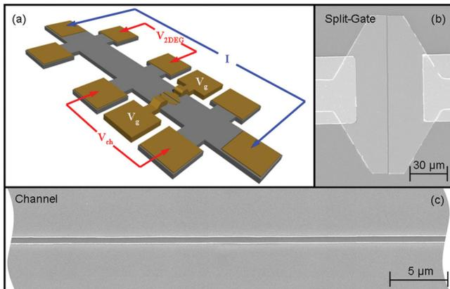
FIG. 1 (color). (a) Schematic diagram of the device's geometry. (b) SEM image of the split-gate structure. (c) Magnified image of the split-gate defined quantum wire.
