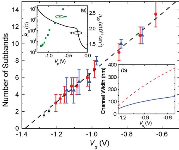
FIG. 3 (color). Number of subbands (channels) in the wire vs gate voltage  $V_g$ . Arrows indicate position of  $V_g = -1245$  mV and  $V_g = -1265$  mV. Inset (a): resistance of wire (left axis) and electron concentration (right axis) vs  $V_g$ . Inset (b): Channel width determined from  $n(V_g)$  for both the parabolic (solid blue line) and square-well (dashed red line) model potentials vs  $V_g$ .
