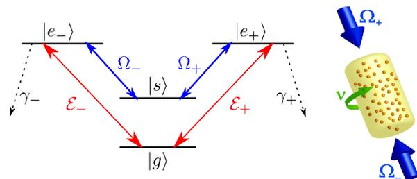
FIG. 1 (color online). The Raman interaction of two counter-propagating control lasers of Rabi frequencies  $\Omega_{\pm}$  and opposite circular polarization coupling to the  $|s\rangle - |e_{\pm}\rangle$  transitions of a double- $\Lambda$  system generates a quasistationary pattern of Stokes fields  $\mathcal{E}_{\pm}$ , called stationary light.
