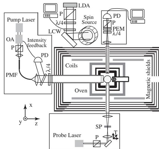
FIG. 1. Experimental setup. PD: photodiode, SP: stress plate to control polarization of the probe beam, T: translation stage to shift the probe beam, P: polarizer, PMF: polarization maintaining fiber, OA: optical amplifier, LCW: liquid crystal wave plate, PEM: photoelastic modulator,  $\lambda/4$ : quarter-wave plate, LDA: laser diode array.
