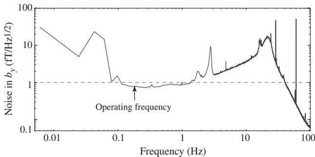
FIG. 2. Frequency spectrum of the comagnetometer noise in measurement of  $b_y^n$ . The broad peak at 20 Hz is the resonance of the coupled spin ensemble, peaks at 2 and 3 Hz are due to mechanical resonances of the floating optical table, and the peak at 0.05 Hz is due to the cycle time of a cooling system.
