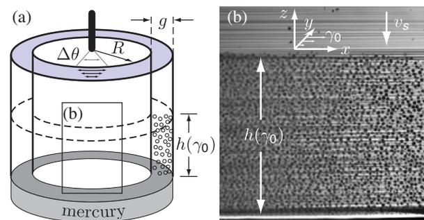
FIG. 1 (color online). (a) Setup for viscous resuspension under oscillatory shear in a Couette geometry. For a strain amplitude  $\gamma_0 = R\Delta\theta/2g$ , the suspension bed rises to a height  $h(\gamma_0)$ . (b) The picture shows particles located in the plane of a laser sheet shined tangentially through the gap of a transparent Couette cell. Horizontal stripes are artifacts caused by imperfect matching of particle and fluid refractive indices.
