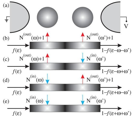
FIG. 2 (color online). (a) The single electron two-islands' circuit. (b)–(e) Diagrams describing the forward inelastic cotunneling rate. The “up” arrows stand for the  $e$ - $h$  pairs excited during the cotunneling and the “down” arrows correspond to the recombination of the  $e$ - $h$  pairs. The vertices shown by boxes are proportional to the probability of an elemental  $e$ - $h$  pair excitation,  $\rho(\omega)/\omega$ .
