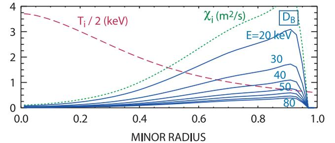
FIG. 4 (color online).  $T_i$  (dashed line),  $\chi_i$  (dotted line), and  $D_B(E, \rho)$  (solid line) used by NUBEAM versus  $\rho$  for the 7.2 MW discharge.
