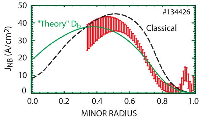
FIG. 2 (color online). Measured beam-driven current (symbols), classical prediction (dashed line), and theory-based prediction (solid line) versus  $\rho$  for the 7.2 MW discharge.
