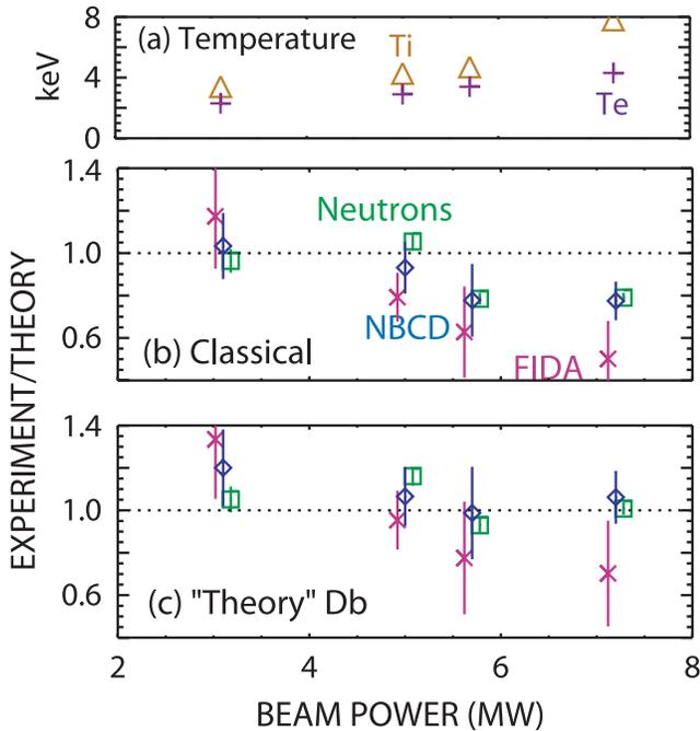
FIG. 3 (color online). (a) Central temperature versus  $P_B$ . (b), (c) Measured neutron rate ( $\square$ ), total beam-driven current ( $\diamond$ ), and FIDA radiance from  $E_\lambda = 20\text{--}60$  keV at  $\rho \approx 0.5$  ( $\times$ ) divided by the classical prediction (b) and by the theory-based prediction (c) versus  $P_B$ .
