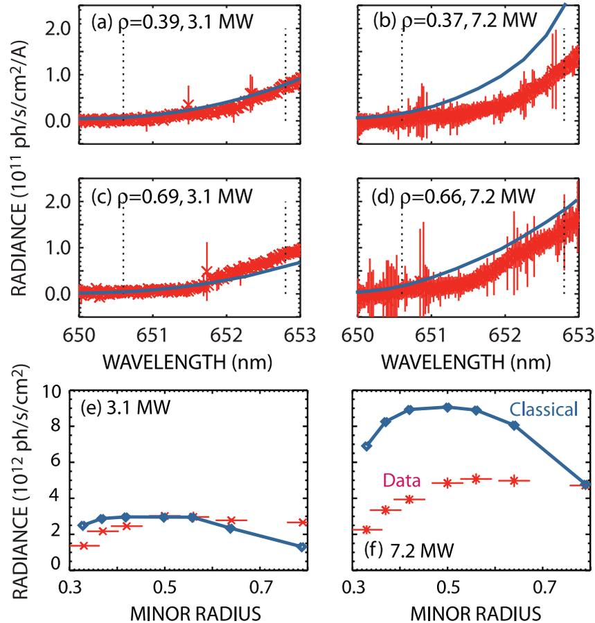
FIG. 1 (color online). (a)–(d) Blueshifted FIDA spectra for two radii and two beam powers. The solid lines are the classical predictions. The dotted vertical lines indicate the spectral band used for the radial profiles. The minor radius  $\rho$  is the normalized square root of the toroidal flux. (e), (f) Radial profile of the FIDA radiance at moderate and high beam power.
